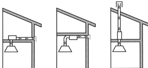
Basing on the chosen direction it is necessary to change position of the air inlet flange with the cover.
