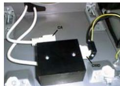
Place the cover of the casing making sure that the holes are coinciding to each other. Fix the cover with the screws supplied with the kit.
