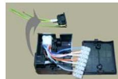
Connect the wires of the blower cable to the terminal board of the junction box respecting the order of colours and the number of wires. The excess of wires can be eliminated or connect in to the terminal board where there aren't wires.
